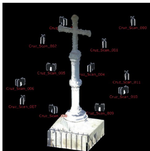
Figure 2. Positions for registering the structure and creating a 3D view of the point cloud. Luis Pinto, 2019.
